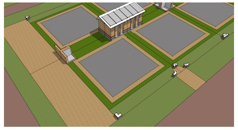
The Plot Module: Wash areas & toilets (rear), and plot corner & entry (front). The toilets are common and house solar panels for the houses.
