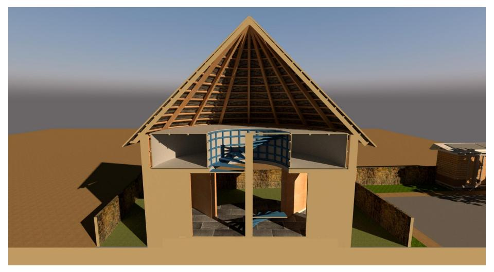
Section through the Water Tank – cutting through shear support walls
