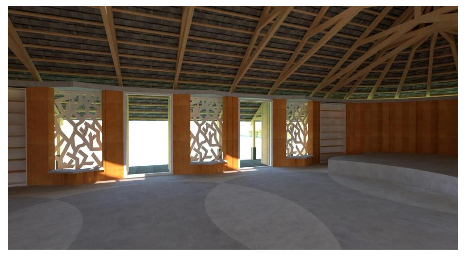
Two double doors on either side open to east (entry) and west (hills). The jaalis provide diffused light cutting out harsh glare.
