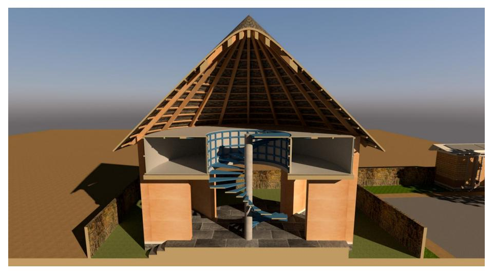
Section through the Water Tank – cutting adjacent to the shear support walls
